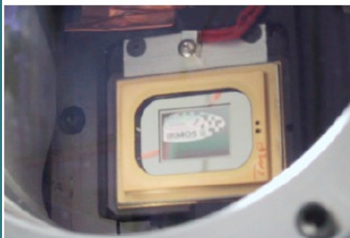
Figure 8: Texas Instruments DMD in test dewar operating at -50C in IRMOS custom socket (without baffle). Note Lakeshore thermal diode mounted at top.
