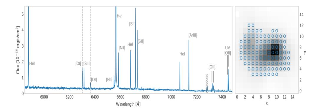
2<sup>nd</sup> order UV [OII] "contamination" because no UV-blocking filter
