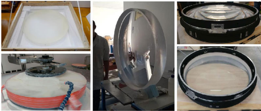
Figure: Current Status of the MOONS (ESO) FC lenses at Officina Stellare where they are being manufactured and integrated in the FC barrel.
