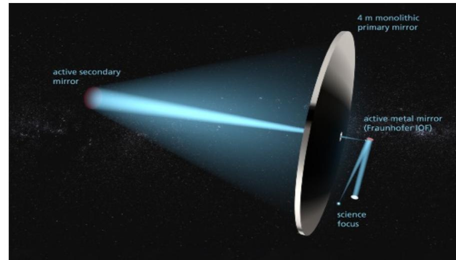
*STOIC concept with 4m monolithic mirror and active deformable mirrors © Fraunhofer IOF*
